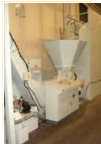
Crusher capacity: 1000 kg/h for cast iron
