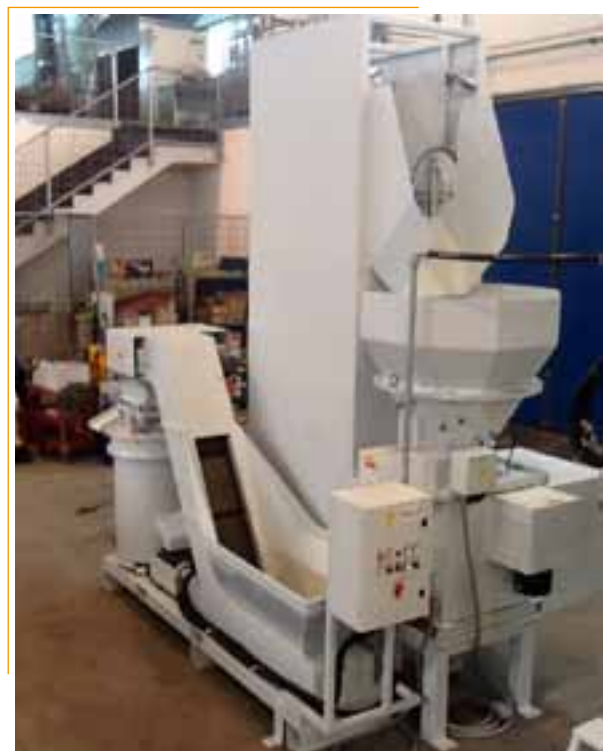
Minisystem with crusher and turner skipoist
