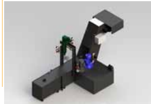
Drag conveyor equipped with drum and self cleaning filter
