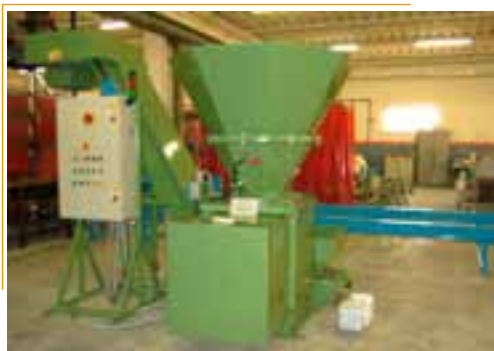
Crusher capacity: 800-1000 kg/h for steel
