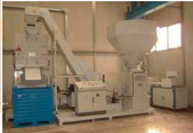
Crusher SCR25 + centrifuge SCE30 800 kg/h for stainless steel - Inconel
