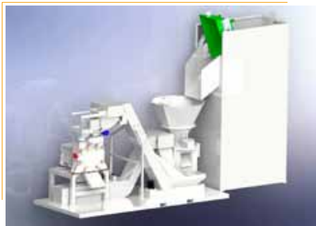
System with turner skiphoist and crusher
