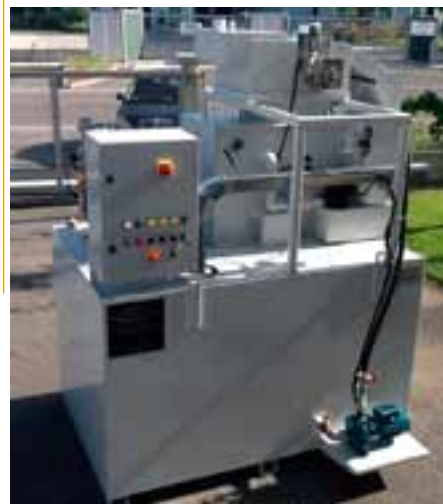
Filtration systems for coolant coming from grinding machines and machining centers
