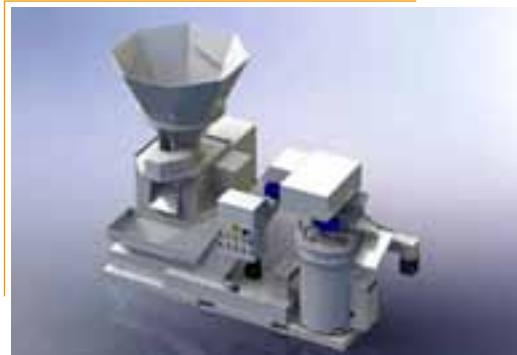
Minisystem with hopper 500 lt + crusher and vibrating screen
