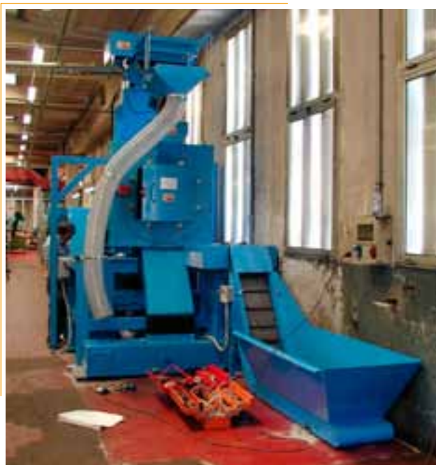
Centrifuge SCE30 1500 kg/h for brass
